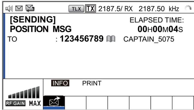
After the call has been sent, the WAIT FOR ACK screen appears as below. The elapsed time since sending the call is displayed.
