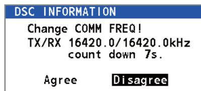
Rotate the **ENTER** knob to select [Agree] then push the knob. The radiotelephone automatically sets working frequency.
